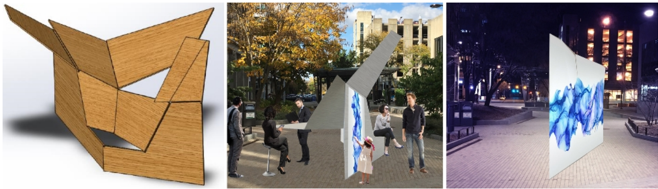
Fig. 9: A case study of the vertex pop-up mechanism, transFORM (three configurations shown above) is 2.5m (approx. 8ft) tall in its flattened configuration (the right-most image, shown at night). The pop-up mechanism constitutes the bottom-most four panels.
